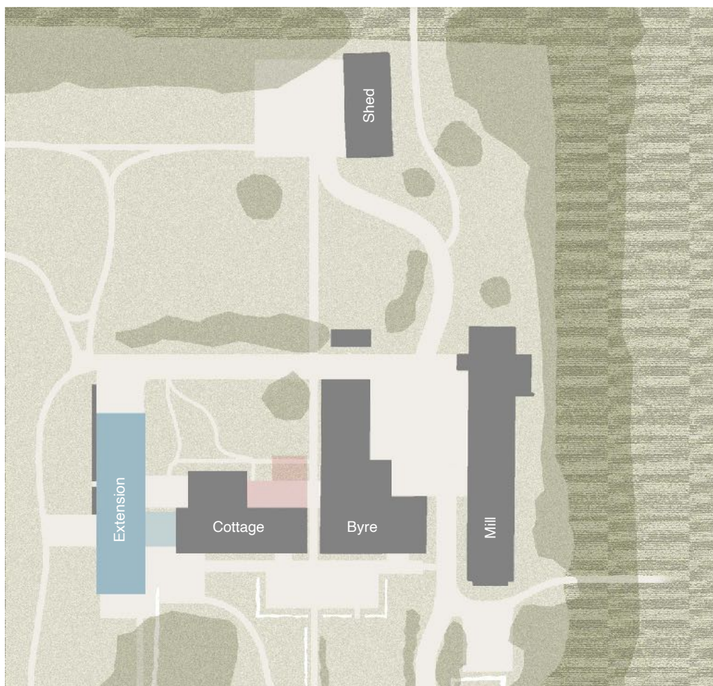
Fig. 7 - Proposed site plan sketch showing cottage NE wing removal and extension.
